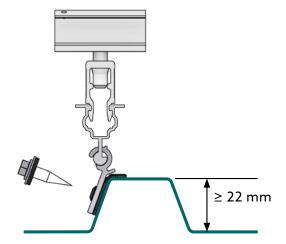
Trapezoidal sheets with minimum height of the side edges: 22 mm
