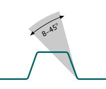
Inclination of the side edges from 8 to  $45^\circ$
